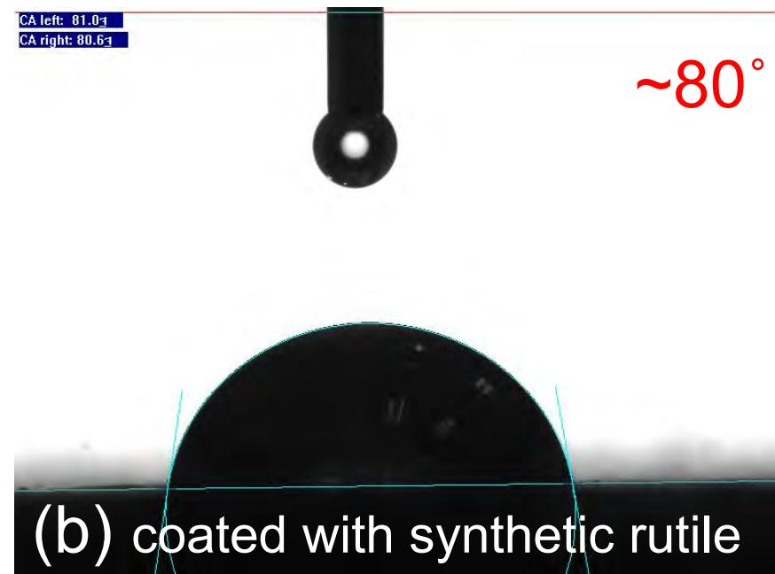
Contact angle measurement for hydrophilic and hydrophobic testing on (a) uncoated and (b) coated ceramic tile under non-irradiation.
