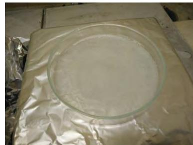
Poured 10 ml of the solution on petri dish and dry at 40 °C
