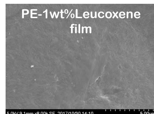
SEM images of PE films with synthetic-rutile/anatase  $\text{TiO}_2$  nanocomposite loading after Xe lamp irradiation for 50 h
